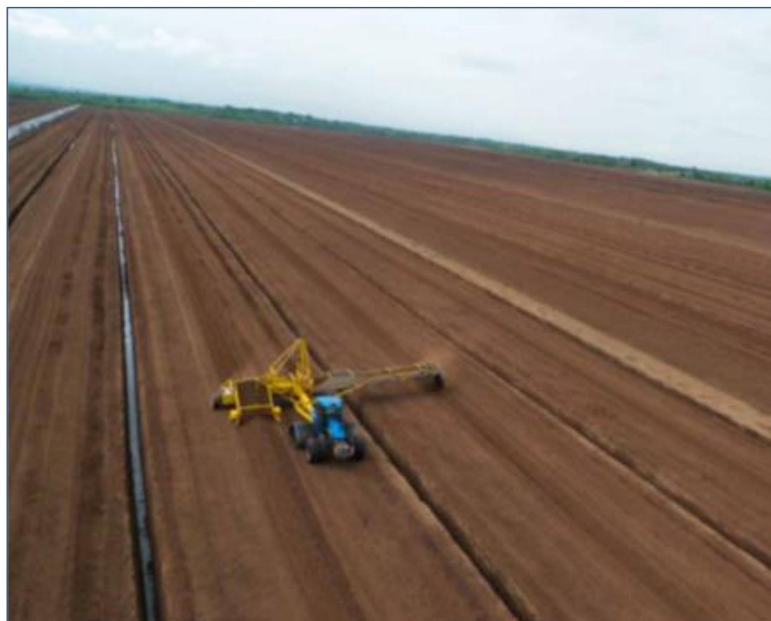
Plate 4-13 Harvesting -Peco method. Image: Bord na Móna
