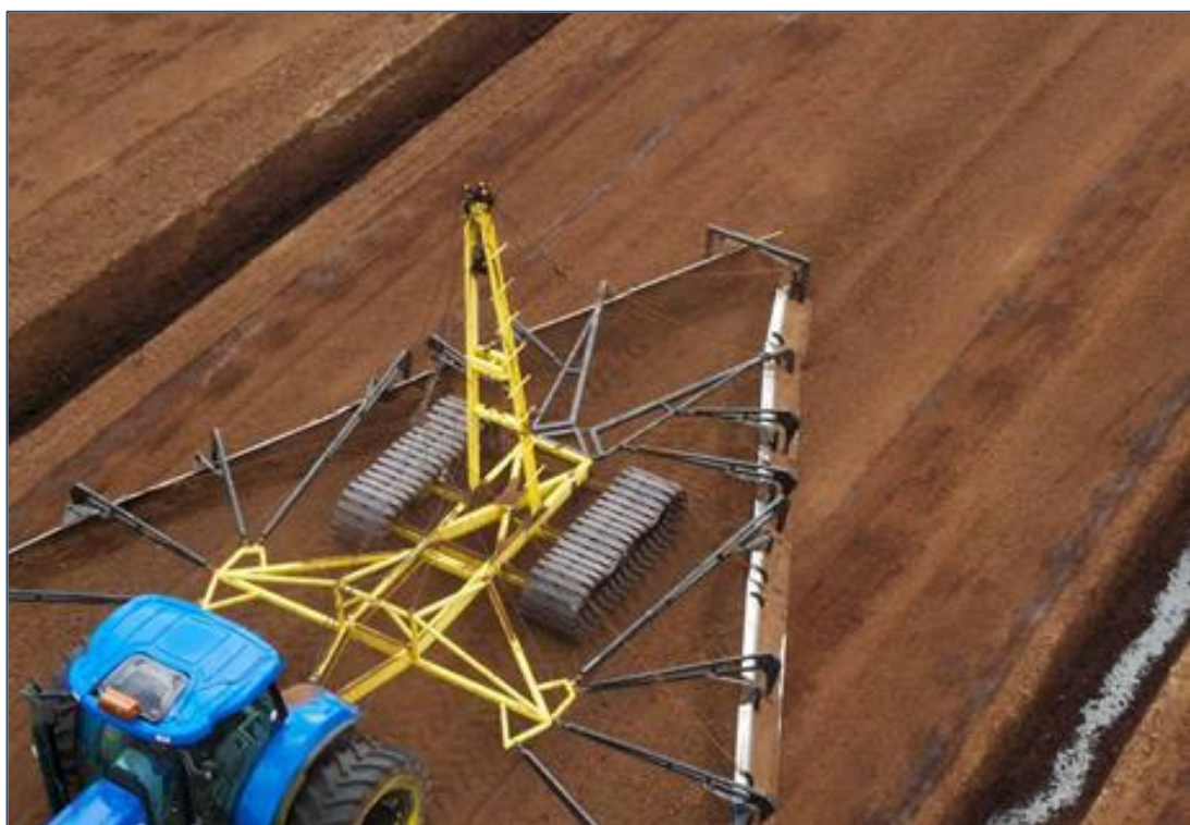
Plate 4-10 Ridging process. Image: Bord na Móna
