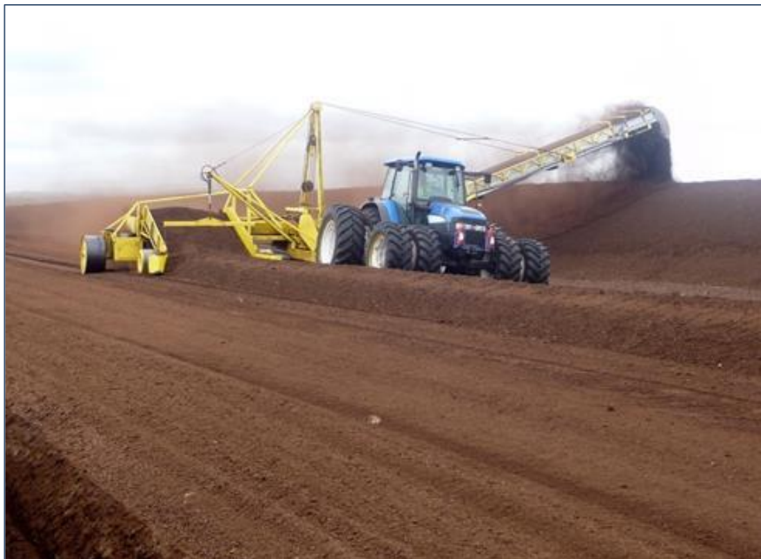
Plate 4-12 Harvesting -Peco method. Image: Bord na Móna
