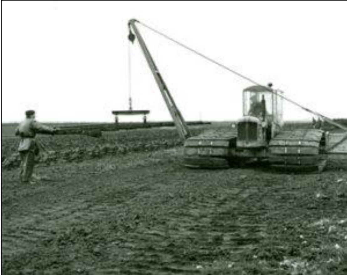
Plate 4-35 Rail Moving Attachment to lift and lay temporary railway track, along Sod Peat ricks and milled peat piles. Source: https://www.bordnamonalivinghistory.ie/equipment-detail/rail-moving-attachment/
